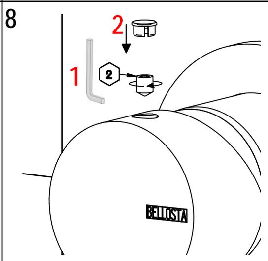
**! SOSTITUZIONE AERATORE/ AERATOR REPLACEMENT**
